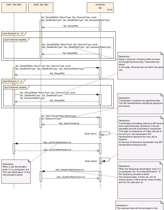
The received data will be allocated in the configured receive buffers, and can be read using the read function for IB Channels.
