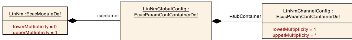
Figure 10-1 LinNm top level configuration overview
