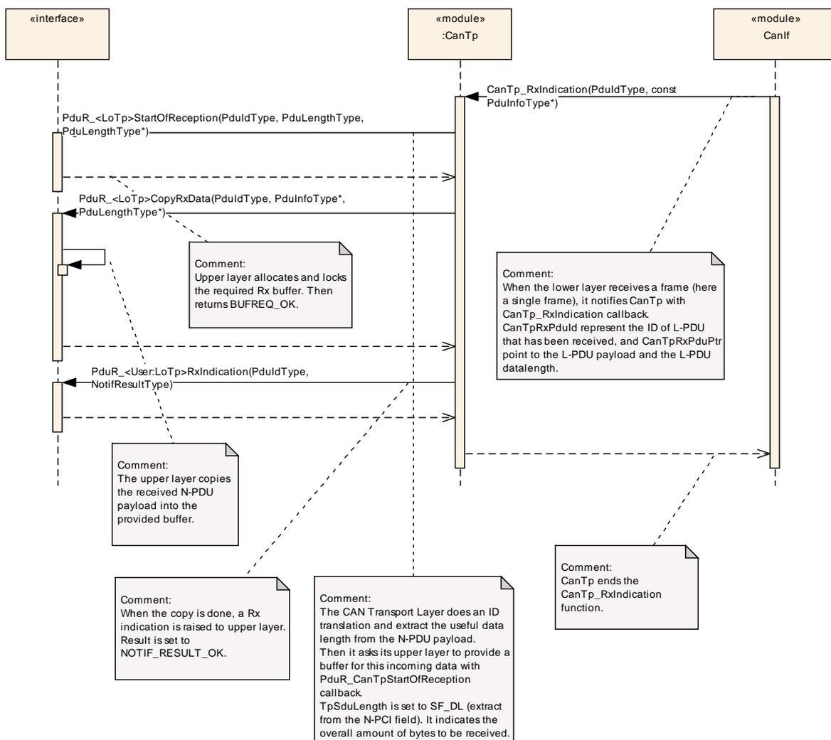
**Note:** This sequence diagram demonstrates the working of the CAN\_Tp module only. However, if the whole system is considered during such reception, more modules are involved. Since this reception can be triggered in the context of CAN ISR, the CAN\_Tp operation should be as short as possible.
