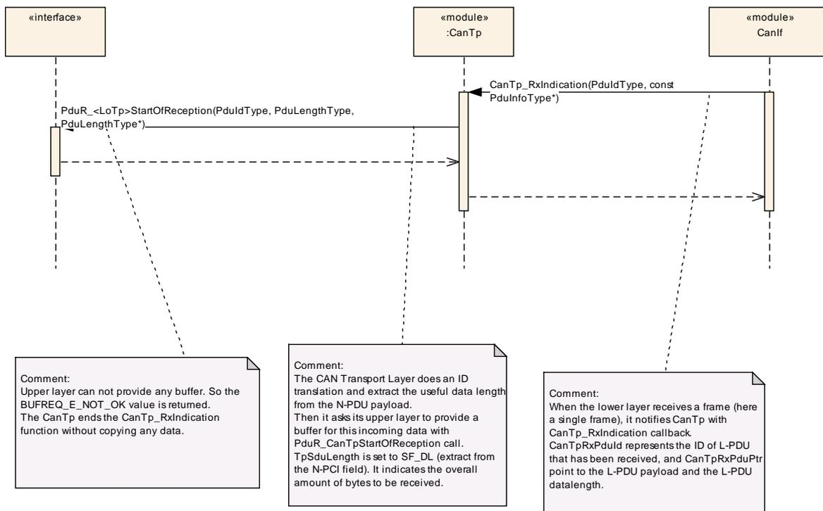
**Note:** This sequence diagram demonstrates the working of the CAN\_Tp module only. However, if the whole system is considered during such reception, more modules are involved. Since this reception can be triggered in the context of CAN ISR, the CAN\_Tp operation should be as short as possible.
