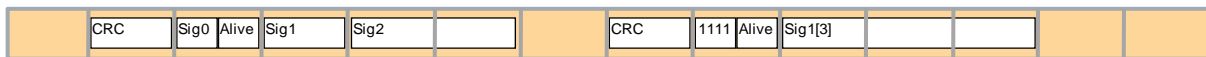
Figure 8-4: E2E Profile 1 example layout (two signal groups protected by E2E in one I-PDU)
