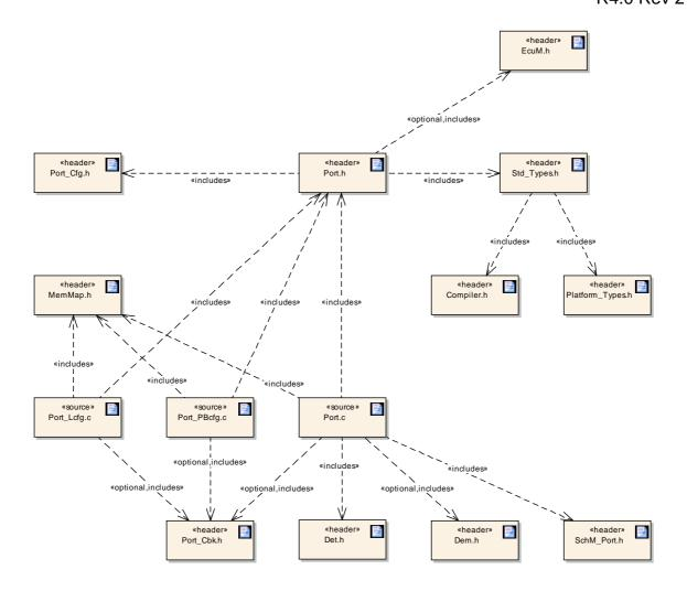
Figure 1 Header File Structure
