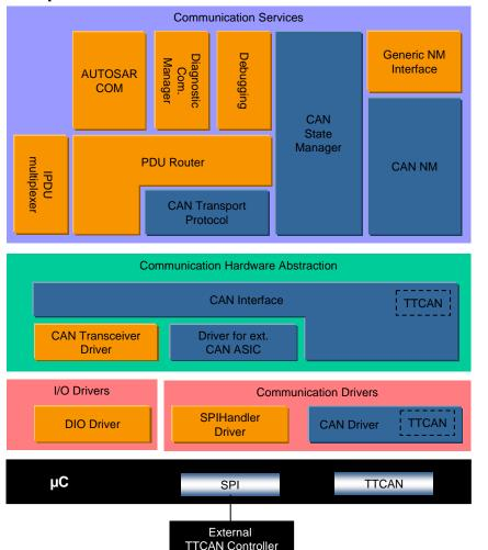
The **TTCAN Communication Services** are the optional extensions of the plain CAN Interface and CAN Driver module for vehicle
