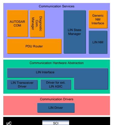
The **LIN Communication Services** are a group of modules for vehicle network communication with the communication system LIN.
