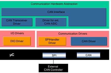
The **CAN Communication Services** are a group of modules for vehicle network communication with the communication system CAN.
