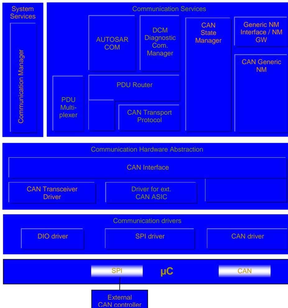
Figure 1 AUTOSAR CAN Layer Model (see [1])
