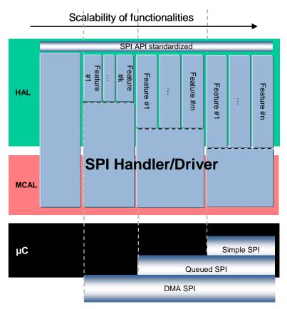
The functional perimeter of this software module will be statically configurable to fit as far as possible to the real needs of each ECU. That means for instance synchronous, asynchronous or both SPI access could be present in the ECU. Consequently, two
