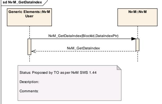
A sequence diagram titled 'sd NvM_GetDataIndex'. It shows two participants: 'Generic Elements::NvM User' and 'Nv M::Nv M'. A synchronous message 'NvM_GetDataIndex(BlockId,DataIndexPtr)' is sent from the user to the Nv M object. A return message 'NvM_GetDataIndex' is received by the user. Below the diagram is a note: 'Status: Proposed by TO as per NvM SWS 1.44' and 'Description: Comments:'. |
