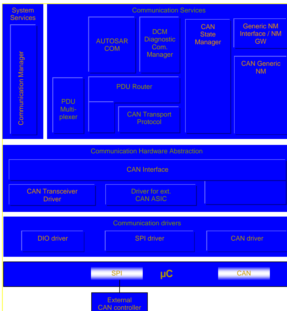
Figure 1 AUTOSAR CAN Layer Model (see [1])
