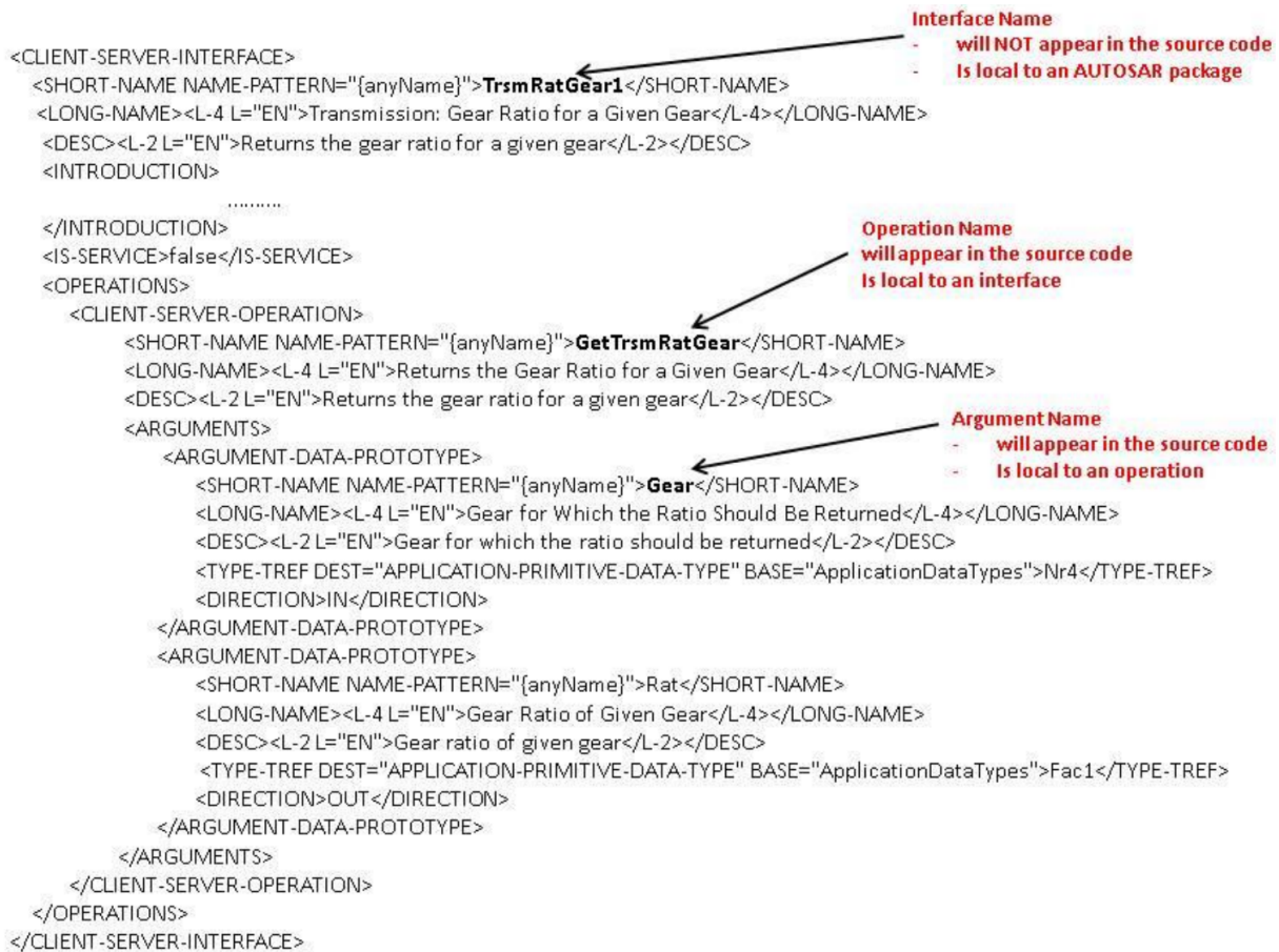
Figure 6.3: ClientServerInterfaces and Operations
