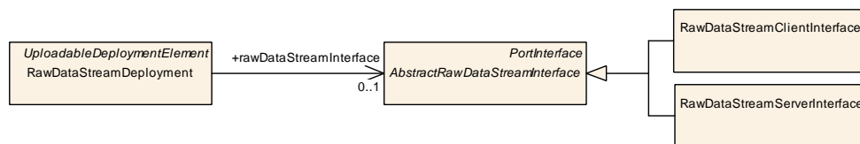
Figure 12.1: Modeling of the RawDataStreamDeployment
