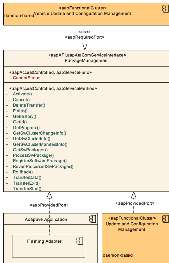
Figure 5.3: Interfaces required by Vehicle Update and Configuration Management from Update and Configuration Management
