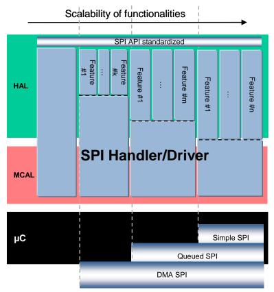
The functional perimeter of this software module will be statically configurable to fit as far as possible to the real needs of each ECU. That means for instance synchronous, asynchronous or both SPI access could be present in the ECU. Consequently, two SPI drivers could exist but just one handler interface. This chapter contains common requirements that are valid both for synchronous and asynchronous SPI drivers.
