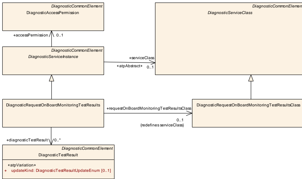
Figure 5.35: Modeling of diagnostic service for OBD Mode 0x06
