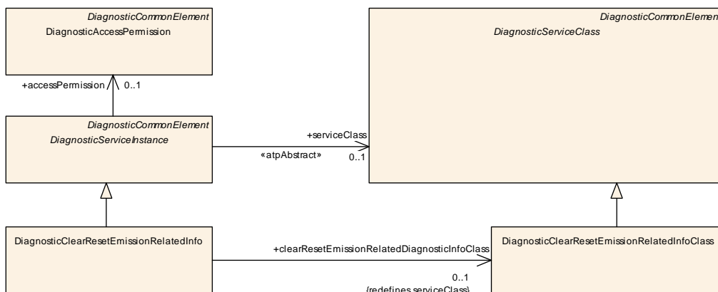
Figure 5.34: Modeling of diagnostic service for OBD Mode 0x04
