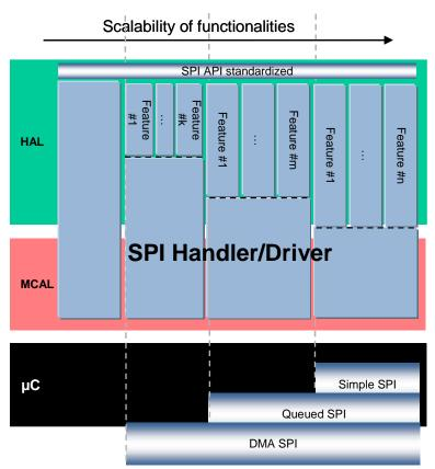
The functional perimeter of this software module will be statically configurable to fit as far as possible to the real needs of each ECU. That means for instance synchronous, asynchronous or both SPI access could be present in the ECU. Consequently, two SPI drivers could exist but just one handler interface. This chapter contains common requirements that are valid both for synchronous and asynchronous SPI drivers.
