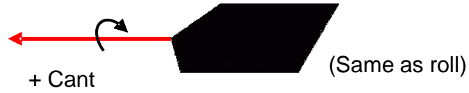
Figure 2.4: Plus, or minus sign of cant
