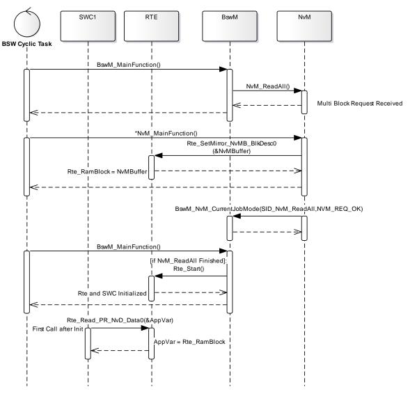
Figure 4: Sequence diagram for Initialization of RAM block
