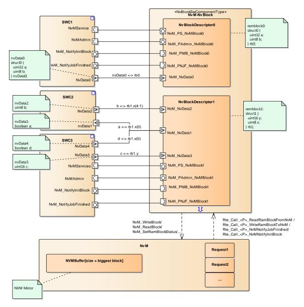
Figure 15: Port configuration for use case 3
