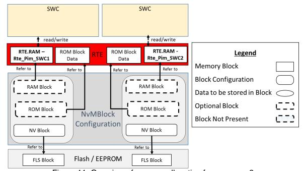
Figure 11: Overview of memory allocation for use case 2
