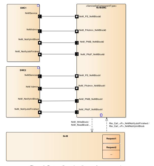
Figure 6: Port configuration diagram for use case 1a
