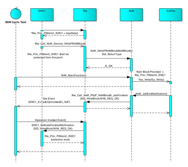
Figure 13: Sequence diagram of NvM access for use case 2
