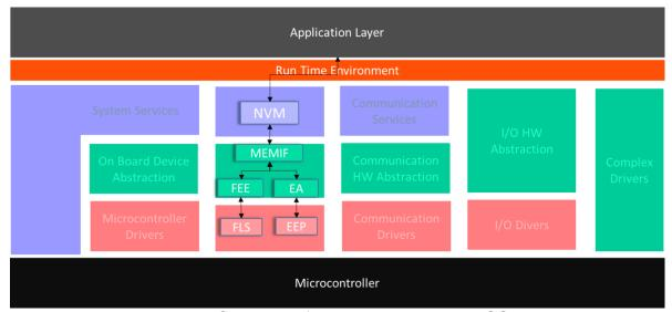
Figure 1: Overview of memory stack in AUTOSAR
