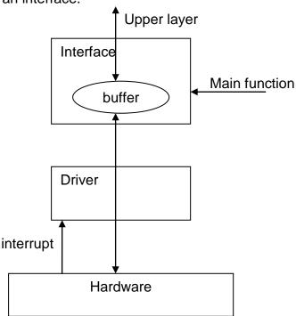
When the Upper layer wants to send data downwards it asks the interface. The interface locks the buffer by suspending all interrupts via the BSW Scheduler, copies
